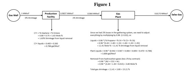
Notice Figure 1 contains the gas stream, shrinkages, shrinkage due to liquid removal (mole % of the liquids removed), shrinkage due to non-hydrocarbon removal and liquid content.
